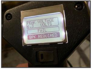
The initial BPK-Probe<sup>™</sup> measurement displayed a FAILED, 6.3 volts on the compressor motor shaft
