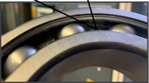
Actual damaged bearing from 243HP Siemens Motor
