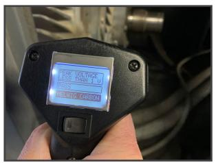
Measurements after the BPK-4 install displayed a PASS, less than 1 volt on the compressor motor shaft
