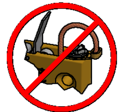
INCORRECT TERMINAL INSTALLATION
