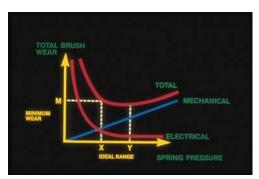
There has always been a fear of applying excess spring force on carbon brushes since that would increase the brush wear rate. On old adjustable spring force holders the instruction was to decrease spring force until there was visible arcing and then increase the force one notch. The recommended spring pressure had been 1.5 to 2.5 PSI depending on the application. The graph shows the relationship between mechanical, electrical,
