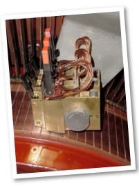
show the amount of wear left while the machine is running.
