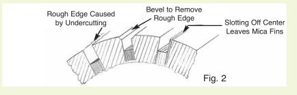
In addition to leaving a jagged edge projecting from the commutator bar, the edge of the bar becomes somewhat work-hardened and hence will not wear down uniformly. Therefore, the edges of the bars must be chamfered by using a suitable slotting file or a specialty shaped scraper. \*\* See Martindale slotting scrapers. \*\*
