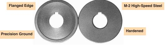
All saws, but especially those which are relatively thin, should be supported with as large as possible diameter flange support washers. These side support washers distribute the clamping force evenly, provide additional stability, and lessen the chance for deflection in thinner blades.
