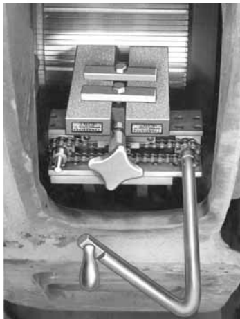
Grinder mounted on Traction Motor
